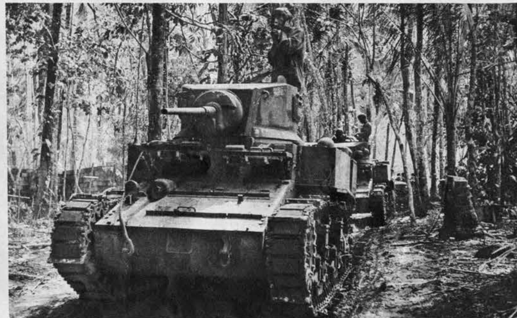
Marines in U. S. M-5's plow through a clearing in the fight for the Munda airfield. M-5 turret has discarded the cupola of the General Stuart, is still cylindrical, with forward slope to its top.
